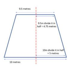
with the southern end of the building and the centre point marked on the floor. A string or laser line can be used to mark this centre line.
