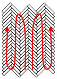
Once all the full boards that can be layed are down, panels that require trimming can then be installed along the walls. Extra space maybe required to manoeuvre panels into place under door frames and architraves.
