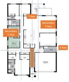
Trowel out enough adhesive to lay out and align the first 2 rows at a time. Ensure that as you layout the flooring along the Y axis that flooring remains aligned as you go. Slight adjustments will need to be made as you go along. Only trowel out small sections of adhesive to avoid adhesive drying out and forming a skin which could reduce adhesion strength. Use the X axis in the same way as to keep alignment of the herringbone pattern.
